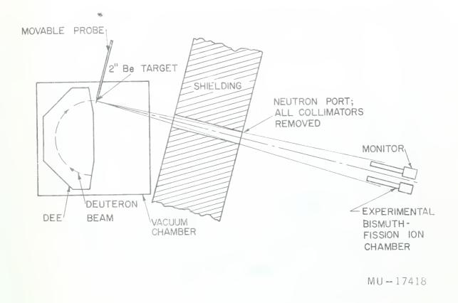
Fig. 8. Schematic diagram of the experimental arrangement at the cyclotron. (Not to scale.)
